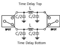
Fig. 4. Schematic of proposed time delay Structure
