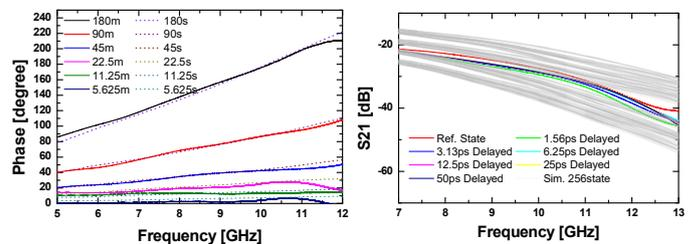
Fig. 7. Measured and Simulated phase state result,  $S_{21}$  of Main bit State
