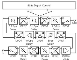
A block diagram of the proposed true time delay circuit
