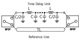
Fig. 2. Schematic of conventional time delay Structure
