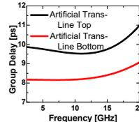
Fig. 5. The simulated group delay error of proposed structure.
