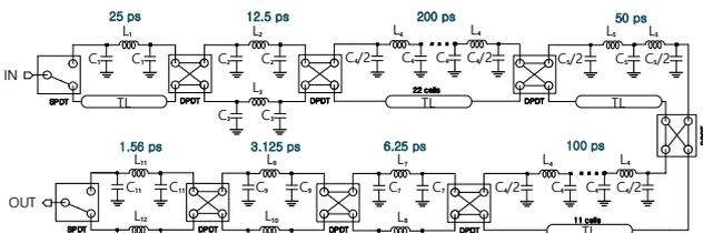
Fig. 1. Schematic of the propose True Time Delay Circuit.
